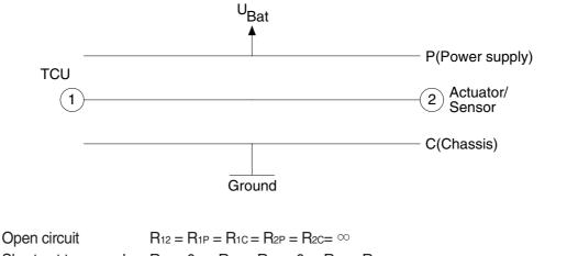
Short cut to ground $R_{12} = 0$ ; $R_{1C} = R_{2C} = 0$ , $R_{1P} = R_{2P} = \infty$ Short cut to battery $R_{12} = 0$ ; $R_{1C} = R_{2C} = 0$ , $R_{1P} = R_{2P} = 0$
