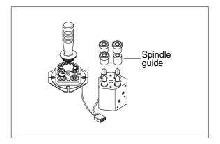
(5) The spindle guides can now be replaced.The O-rings on the spindle guide must be replaced before the valve is reassembled.
