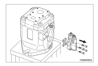
(2) Measure dimension A, B and note down. Check sealing surface (1). Replace gasket (2).
