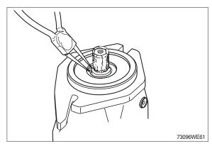
Change the shaft seal and check its sliding surface (drive shaft) and housing, grease the sealing ring.
