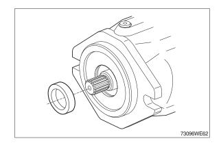
(2) Assembling of the sealing ring carefully down to the stop ring.
