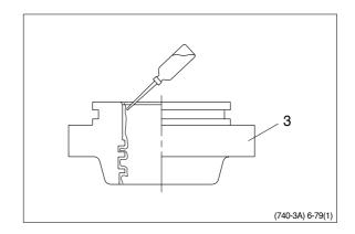
Coat dust wiper(8) with grease and fit dust wiper(8) to the bottom of the hole of dust wiper.
