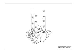
3) Place first spool section(O-ring side up) on inlet section, position O-ring and insert load check poppet(Nose down) and spring(Behind poppet) into load check cavity as shown. Repeat this procedure for each spool section; The load check springs are compressed by the following sections during assembly.
