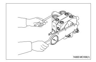
6) Install auxilliary valves and plugs and torque to proper specifications.
