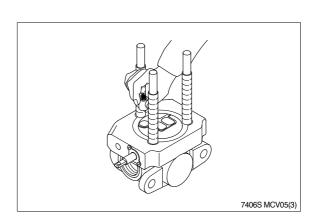
4) Position end section on last spool section as shown and hand tighten tie rod nuts. The end section on picture is a "turn around" section without ports. Universal outlet/power beyond section and power beyond and closed center sections are also used as end sections. These end sections do not have O-ring grooves.
