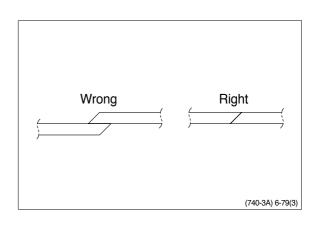
Rod seal(5) has its own fitting direction. Therefore, confirm it before fitting them. Fitting rod seal(5) up side down may damage its lip. Therefore check the correct direction that is shown in fig.
