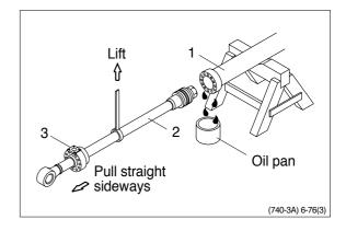
Note that the plated surface of piston rod(2) is to be lifted. For this reason, do not use a wire sling and others that may damage it, but use a strong cloth belt or a rope.
