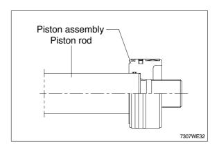
Tighten nylon nut(18) to piston rod(2) Tightening torque
