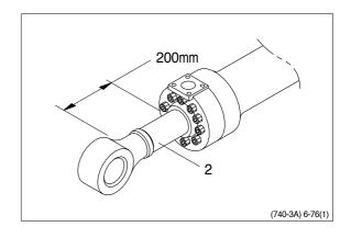
Loosen and remove socket bolts(19) of the gland(3) in sequence.
