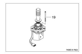
(3) The upper portion of the valve, from the mounting plate upwards, can now be detached and placed to one side.
