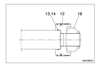
Remove the gland assembly from piston rod(2).
