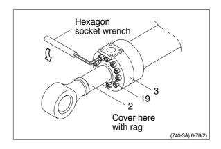
Draw out gland(3) and piston rod (2) assembly together from cylinder tube(1). Since the piston rod assembly is heavy in this case, lift the tip of the piston rod(2) with a crane or some means and draw it out. However, when piston rod(2) has been drawn out to approximately two thirds of its length, lift it in its center to draw it completely.
