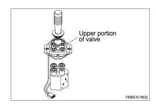
(4) Remove the ball carriers off of the spindle guide - carefully detach the spindle guides, being careful to ensure that no contamination enters the valve.
