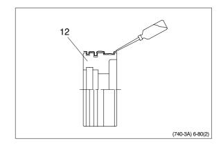
Fit piston seal(15) to piston
