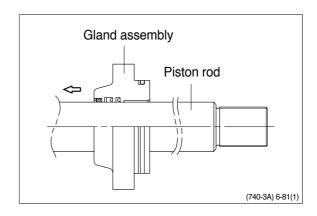
Fit piston assembly to piston rod.
