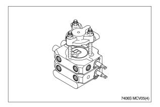
5) Position valve assembly with the mounting pads of the end sections on a flat surface. To obtain proper alignment of end sections relative to the spool sections apply downward pressure to the end sections; Snug tie rod nuts to about 10lbf · ft. Final torque the two 11/16 nuts to 48 ± 5lbf · ft; Final torque the 3/4 nut to 74 ± 8lbf · ft. Check for proper spool movement.
