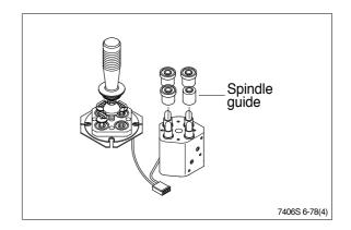
(5) The spindle guides can now be replaced.
