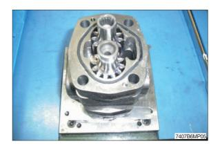
(6) Assemble thrust plate.
