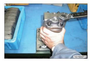
(15) Use torque wrench to assemble.  $\cdot$  Tightening torque : 15 kgf  $\cdot$  m (108 lbf  $\cdot$  ft)
