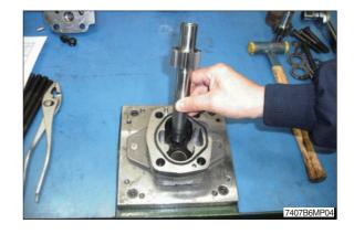
(5) Assemble driven gear. Spread hydraulic fluid around gear set.
