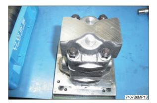
(14) Use air impact to assemble nuts. At this time, assemble nuts diagonally.
