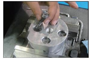
(11) Disassemble plug (2). • Tool : wrench 10 mm
