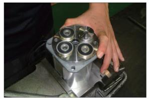
(7) Disassemble magnet (21) and rod stopper (18).
