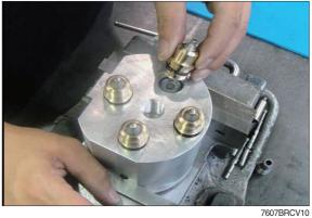
(10) Disassemble spring (4) and spool kit.
