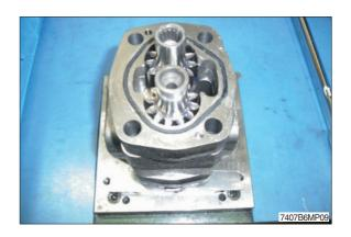
(10) Assemble thrust plate.
