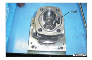
(9) Assemble drive gear set.Spread hydraulic fluid around gear set.
