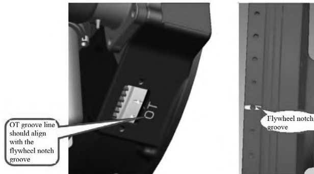
Figure 12 Flywheel notch groove
