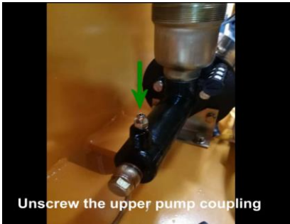
5) Unscrew the upper pump coupling
