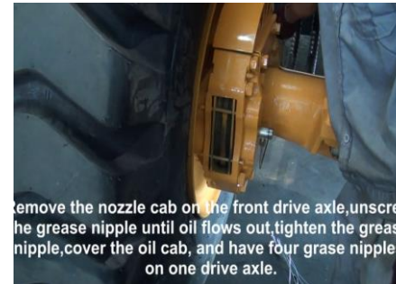
6) Remove the nozzle cap on the front drive axle, unscrew the grease nipple until oil flows out, tighten the grease nipple, cover the oil cap, and have four grease nipples on drive axle.
