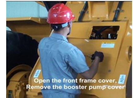
4) Open the front frame cover, remove the booster pump cover
