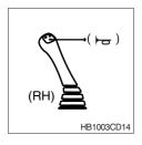
This switch is at the top of right side control lever (backhoe side).
