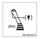
This switch is at the top of right side control lever (backhoe side).
