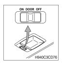
(1) Remove ON/OFF to switch on the cab interior light. Make sure the light is turned off when you intend to leave the machine for a long period of time.
