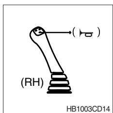
① This switch is at the top of right side control lever (backhoe side).
