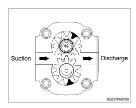
If there is no resistance in the oil passage into which the discharged oil flows, the oil merely flows through the passage, producing no increase in pressure.
