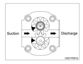
Except for the oil at at the above of the gear teeth, is trapped between the gears teeth, the oil trapped between the gear teeth, is prevented from returning to the suction side with the gears in mesh.
