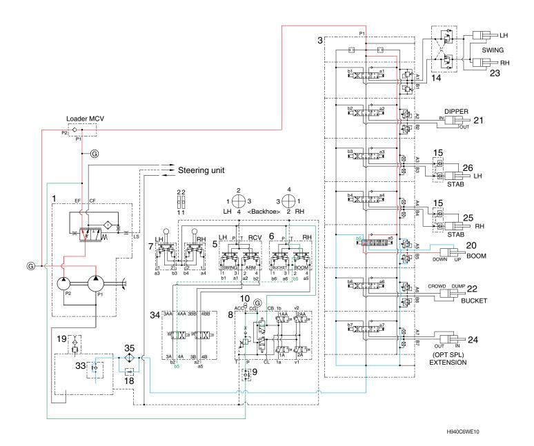
When the backhoe right control lever is pushed forward, the boom spool in the main control valve (3) is moved to the down position by the pilot oil pressure from the remote control valve (6).
