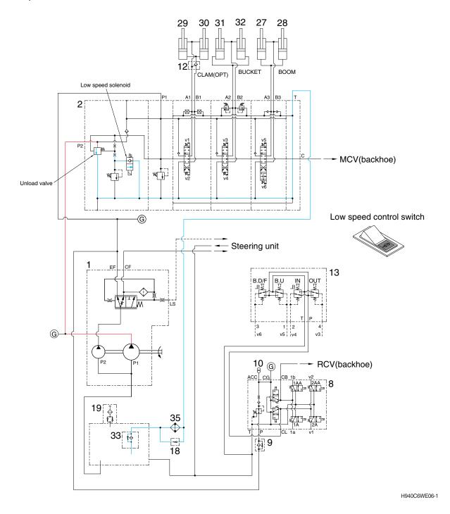
If the low speed control switch is pushed ON, the low speed solenoid is energized.
