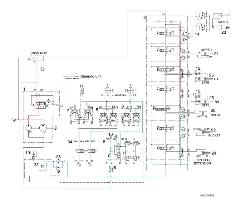
When the backhoe right control lever is pulled back, the boom spool in the main control valve (3) is moved to the up position by the pilot oil pressure from the remote control valve (6).
