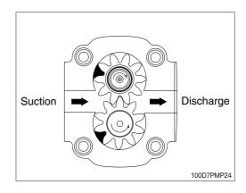
Since the gears are constantly delivering oil, the oil delivered to the discharge port is forced out of the port. The amount of discharge increases with the rotation speed of the gear.
