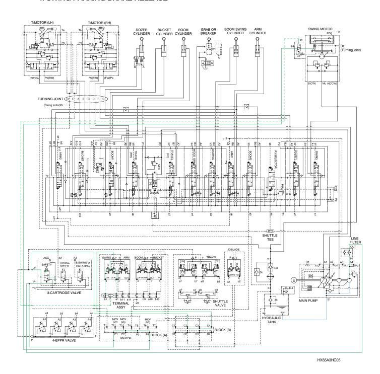
When the swing control lever is tilted, the pilot oil flow into **sh** port of shuttle valve, this pressure move spool so, discharged oil from pilot pump flow into **pg** port.
