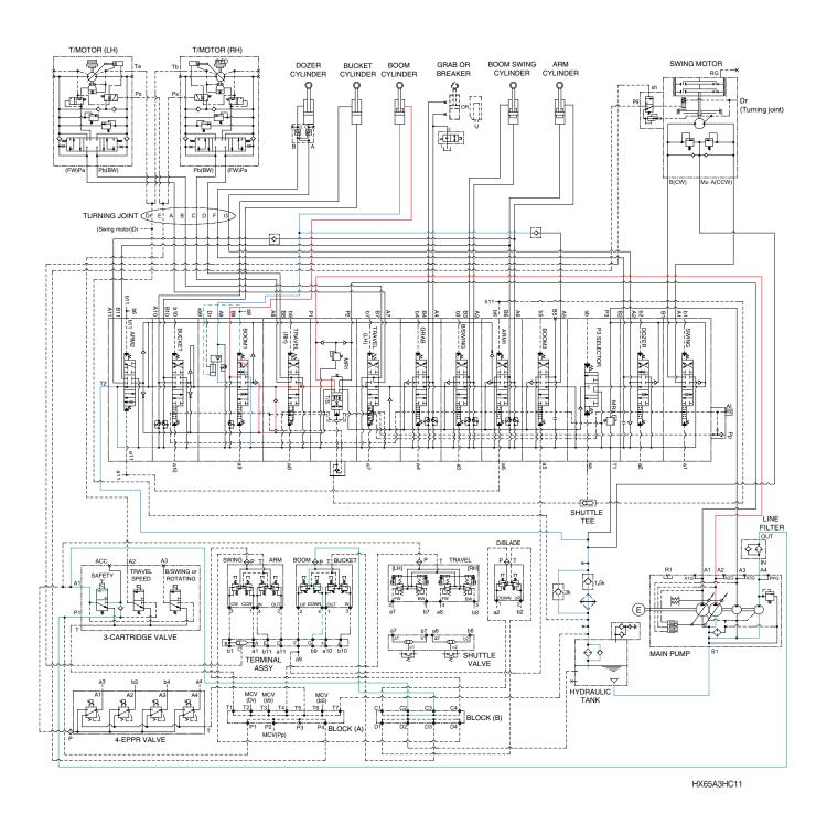
When the right control lever is pushed forward, the boom spool in the main control valve are moved to the down position by the pilot oil pressure (b9) from the remote control valve.
